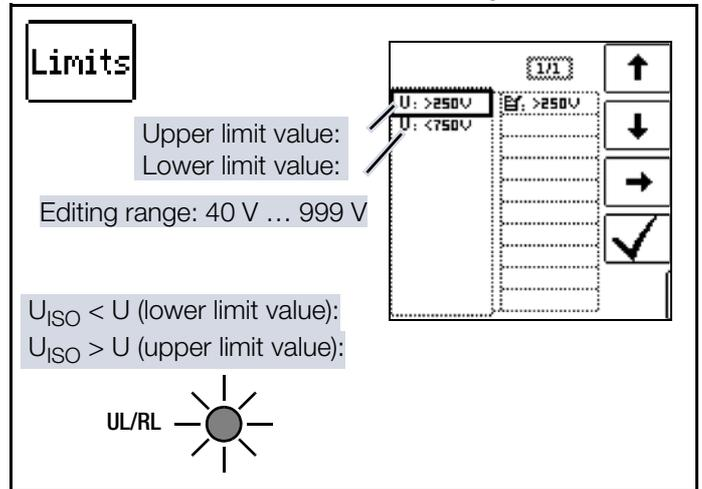
A target range can be defined by setting upper and lower limit values for insulation voltage U<sub>ISO</sub>. If the measured value is not within this range, the UL/RL LED lights up red. An editable value is available for the adjustment of each limit value.
