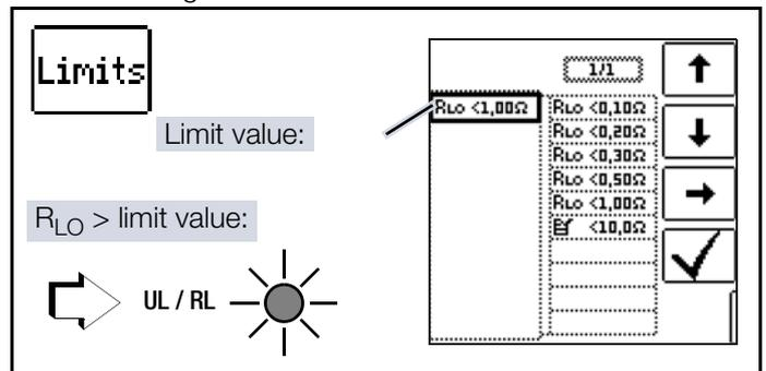
The limit value for resistance can be set as desired. If measured values occur which are above this limit value, the red UL/RL LED lights up. Limit values can be selected within a range of 0.10 Ω to 10.0 Ω (editable). The limit value is displayed above the measured value.
