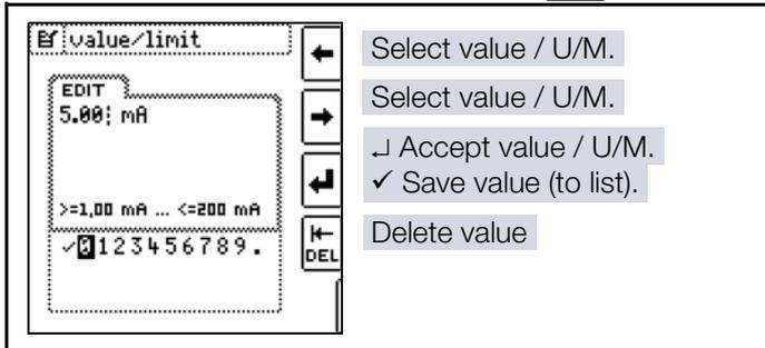
3. Select the respective values with the left or right cursor key. The value is accepted by pressing the  $\downarrow$  key. The value is acknowledged by selecting  $\checkmark$  and then pressing the  $\downarrow$  key. The new parameter is added to the list.
