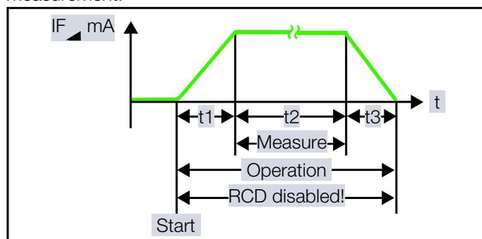
Fig. 6: Suppression of RCD Tripping with Pulsating Current-sensitive RCCBs
