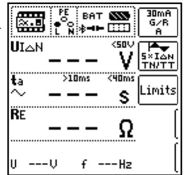
In both cases tripping time must be between 10 and 40 ms (10 ms = minimum delay time for type G RCCBs!).
