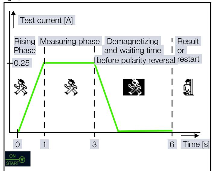
Fig. 5: Representation of Measuring and Waiting Times for Protective Conductor Resistance Measurement at PRCDs
