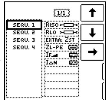
The current test step number appears in the header instead of the memory and battery icons.
