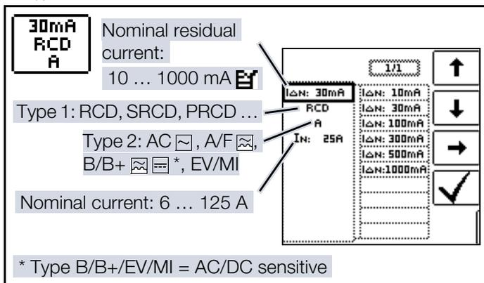
One of the following waveforms can be selected for the test current to be applied:
