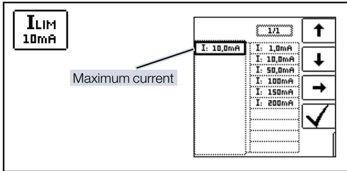
**I<sub>LIM</sub>**: maximum current which may flow before high-voltage is shut down (1 to 200 mA).
