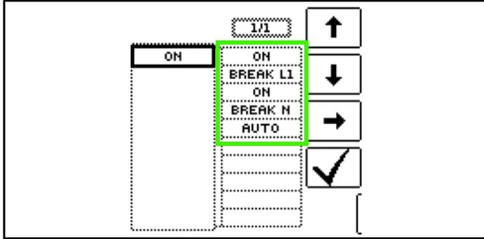
**Semi-Automatic Changing of Fault Simulations/Statuses**
