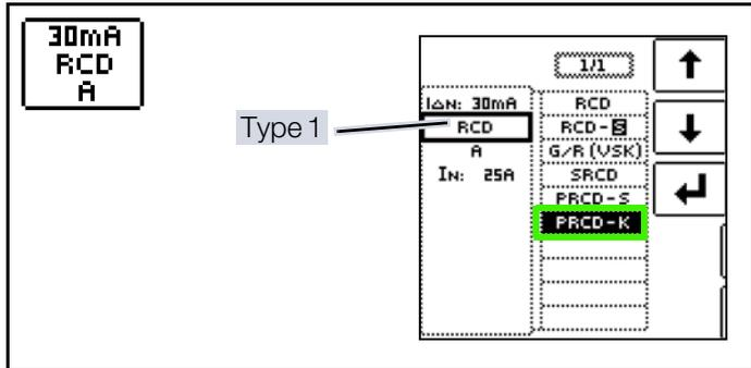
Whether or not PRCDs and selective RCDs are of like design can be tested by measuring touch voltage  $U_{I\Delta N}$ . If a touch voltage  $U_{I\Delta N}$  of greater than 70 V is measured at the PRCD of an otherwise error-free system, the PRCD more than likely contains a non-linear element.
