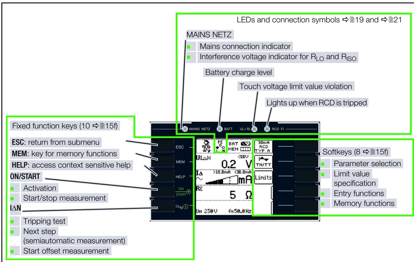
Fig. 3: Control and Display Panel
