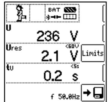
If the voltage threshold is not fallen short of, residual voltage is measured no later than after the selected time has elapsed.
