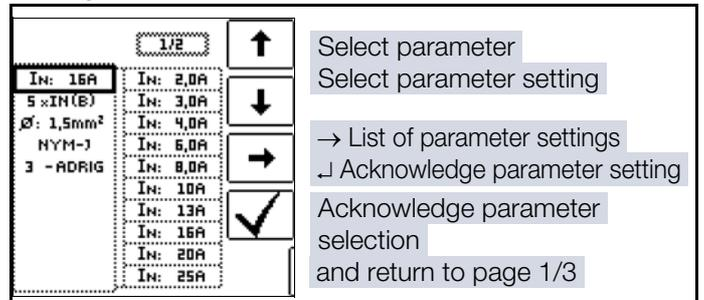
For example, nominal current values must be entered here for the selected electrical circuit. Measuring parameters which have been accepted and saved in this way are subsequently accepted by the current measuring menu automatically when the display is switched from the structure view to measurement.
