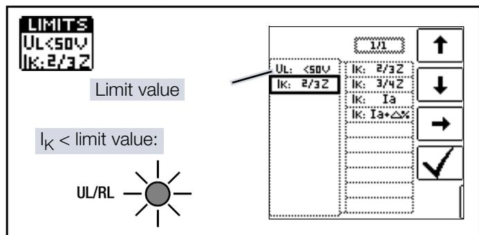
Short-circuit current  $I_K$  is used to test shutdown by means of an overcurrent protective device. In order for an overcurrent protective device to be tripped on time, short-circuit current  $I_K$  must be greater than tripping/breaking current  $I_a$  (see table ⇒ "RCM Display Values" 160).
