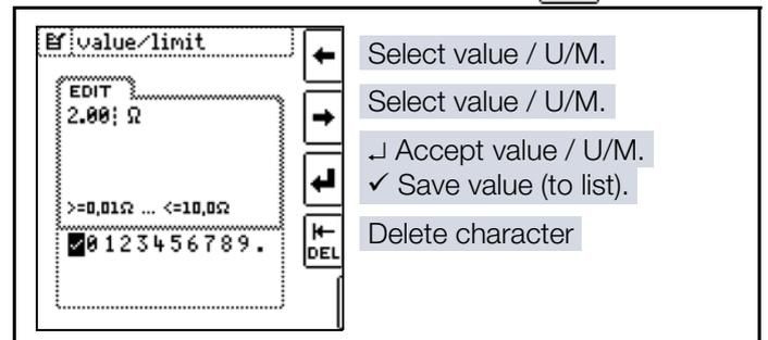
4. Select the respective values with the left or right cursor key. The value is accepted by pressing the  $\downarrow$  key. The value is acknowledged by selecting  $\checkmark$  and then pressing the  $\downarrow$  key.
