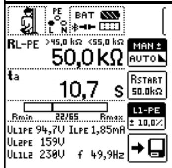
Measurement can be aborted by pressing **ON/START** or **ESC**. The evaluation prompt appears (see above) even after aborting with **ESC**.
