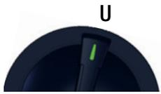
The **U** measuring function provides the opportunity of measuring direct voltage, as well as alternating voltage and its associated frequency.
