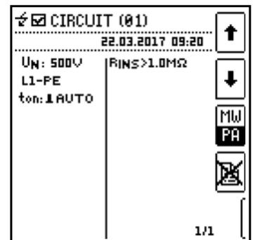
**Viewing, and if Desired Deleting, Stored Measured Values**
