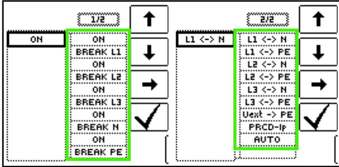
PRCD-K, single-phase: 4 parameters = 4 test steps
