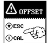
4. Start offset measurement by pressing the triggering key once again ( $I_{\Delta N}$ ), or abort offset measurement by pressing the **ON/START** key (in this case **ESC**).
