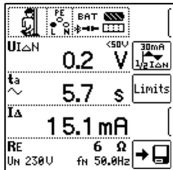
4. After stopping the measurement, the **ok?** evaluation prompt appears and the stopwatch is stopped.
