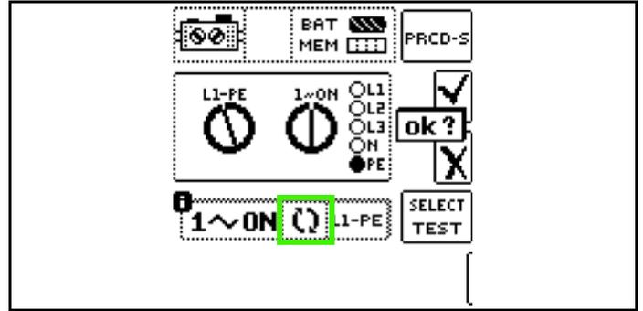
Simulation of PE to phase (step 8):
