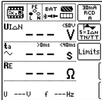
14.6.3 TESTING OF RCCBS WHICH ARE SUITABLE FOR PULSATING RESIDUAL DIRECT CURRENT
