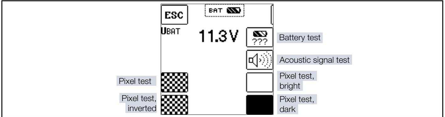
Battery test: battery voltage is displayed, along with charge level as a percentage.
