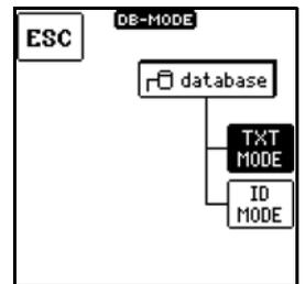
You can work in the ID MODE as an alternative, in which case “ID” appears in the header. You can create structure elements in the measuring/test instrument and label them with any desired ID numbers.
