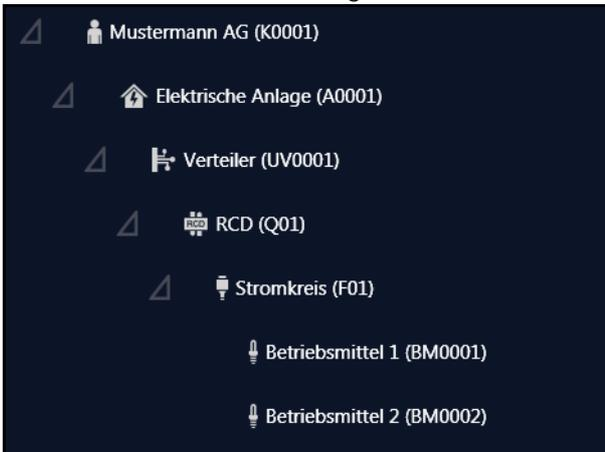
This section describes creation of the distributor structure at the measurement/test instrument.
