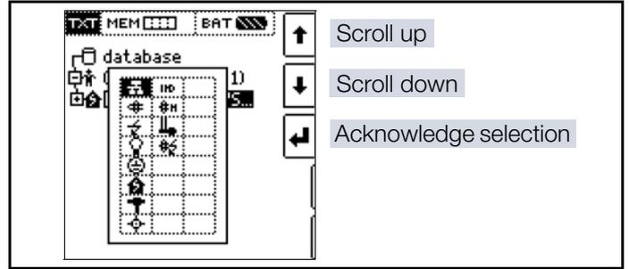
Select the desired object from the list with the ↓ keys and acknowledge with the ↵ key.
