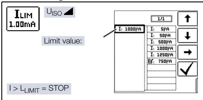
Limit value I<sub>LIM</sub> can be set for the purpose of current monitoring. Measurement is aborted if the limit value is exceeded. Various fixed parameters or an editable value can be selected.
