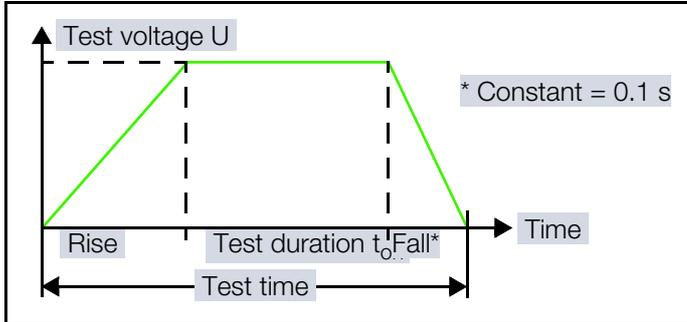
After selected rise time  $t_{\uparrow}$  has elapsed, specified U is applied until the selected test duration  $t_{on}$  has elapsed.
