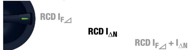
Each of the 3 tripping tests described in the following pages begins with a touch voltage measurement for safety reasons before the actual tripping test is started. Respective maximum touch voltage  $U_L$  must be specified here under limits, which must not be exceeded. If prevailing touch voltage  $U_{I\Delta N}$  is greater than limit value  $U_L$ , safety shutdown ensues.
