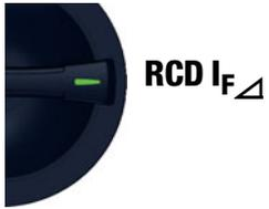
This measuring/test instrument offers the option of testing type B RCDs with smooth direct current.
