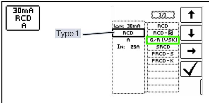
Touch voltage and time to trip can be tested using the RCD – G/R setting.
