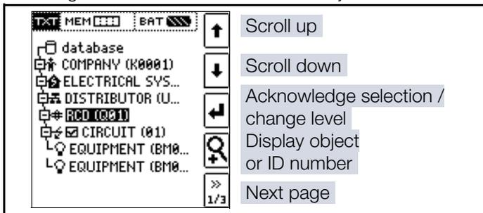
Use the ↓ keys in order to select the desired structure elements.
