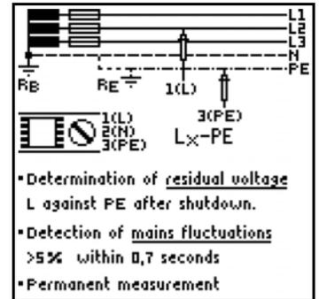
Measurement is continuously active, i.e. voltage dips are automatically detected without pressing a key.
