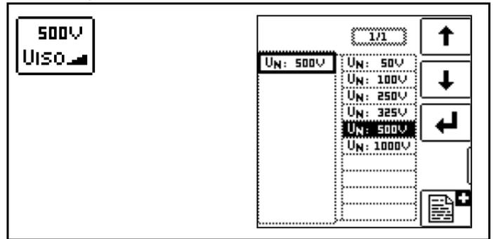
Various preset parameters are available for setting test voltage. The list can be extended with the help of the editing function. This function is made available as soon as the cursor is located in the parameter selection column. See chapter "Freely Selectable Parameter Settings or Limit Values" → 59.
