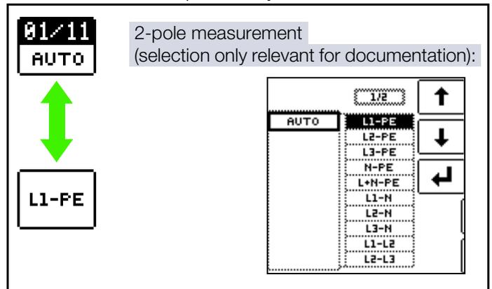
The specification of conductor relationship points makes it possible to allocate measured values and measuring points to each other. Corresponding report generation is possible after measurement has been completed by pressing the save key (softkey).
