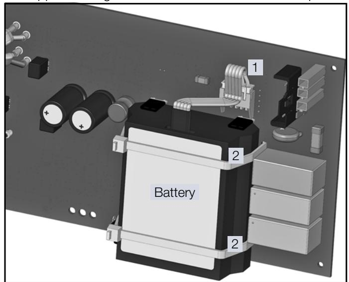
Fig. 9: Screenshot: Removing the Lithium-Ion Battery
