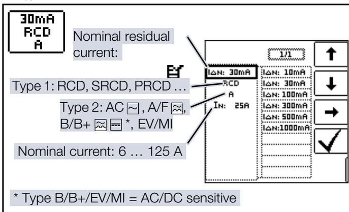
The following parameters can be configured for the test:
