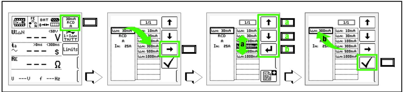
1. Access the submenu for setting the desired parameter.
