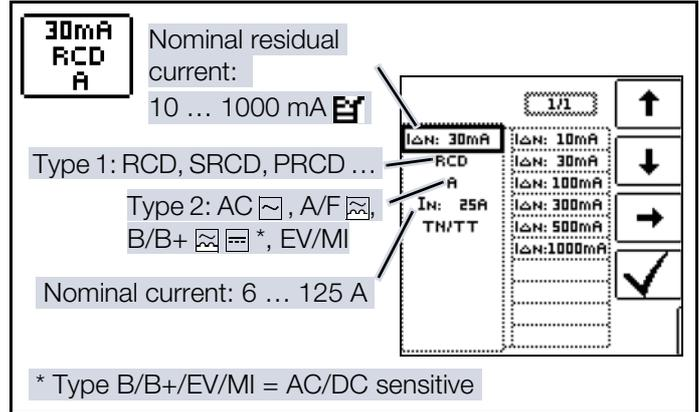
The measuring/test instrument offers the option of displaying limit value violations. The following limit values can be configured:
