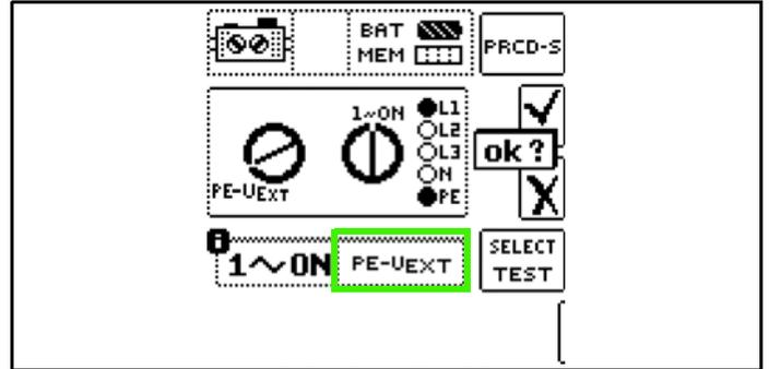
Contact ON key at PRCD with probe (step 10):
