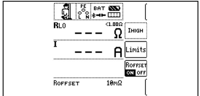
1. Activate the R<sub>OFFSET</sub> function by pressing the corresponding softkey.
